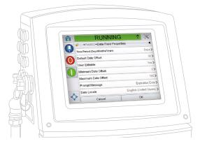
**Foolproof set-up wizardry.** Easily create error-proofing rules during job setup – such as whether or not fields can be edited, permissible data types, date range restrictions and more.
