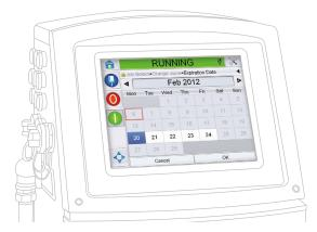
**Multiple choices for minimal errors.** Data-entry screens limit operators to the choices defined during job setup. Entering a date? Choose it from a calendar showing permissible expiration dates. A country code? Choose it from a drop-down list. A lot code? Load it into a predefined format automatically.
